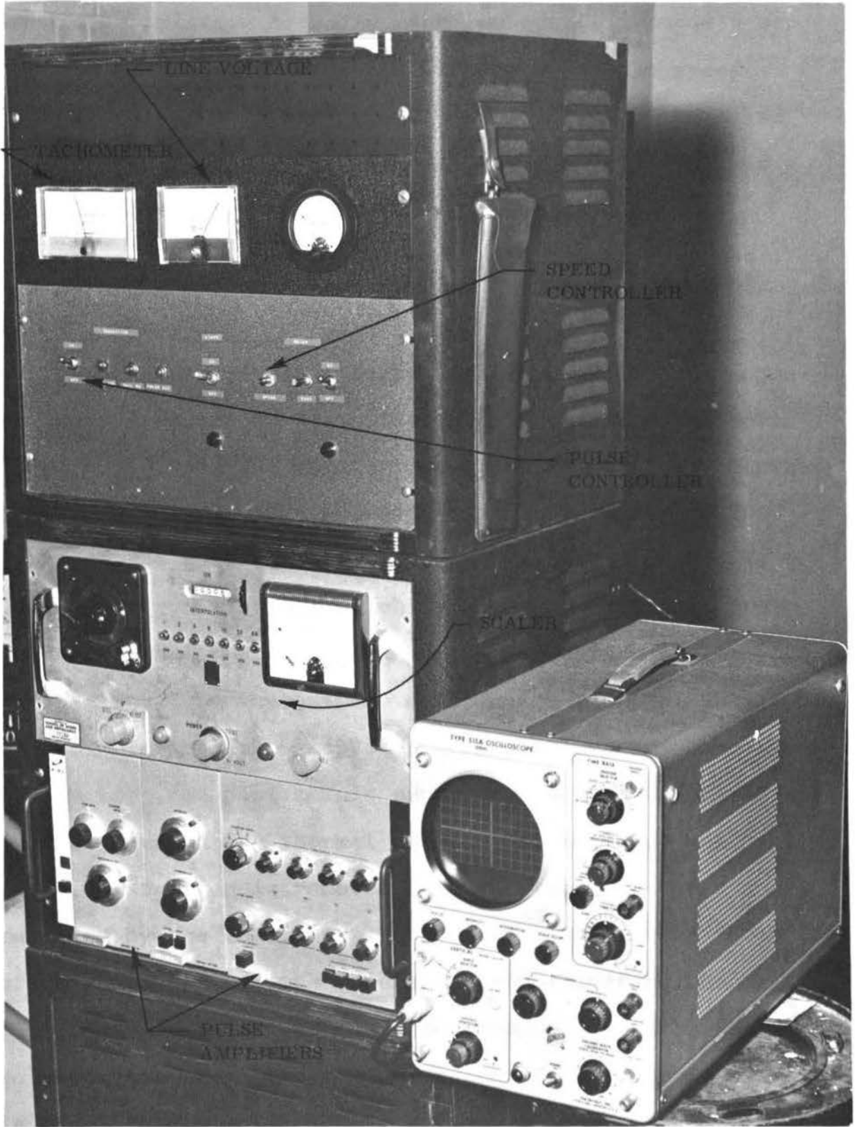
Fig. 9 Neutron Chopper Control Panel
